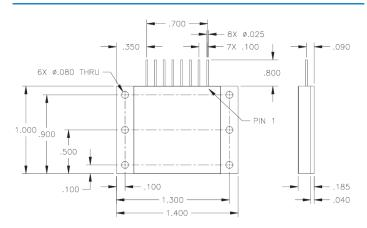
Drawing shows the hermetic package, mounting flange and 8 external connections. All dimensions given are inches, tolerances  $\pm 0.005$ . The package walls are 0.040 inch thick, cover is 0.010 inch thick. Pin 1 is top-right in the diagram.
